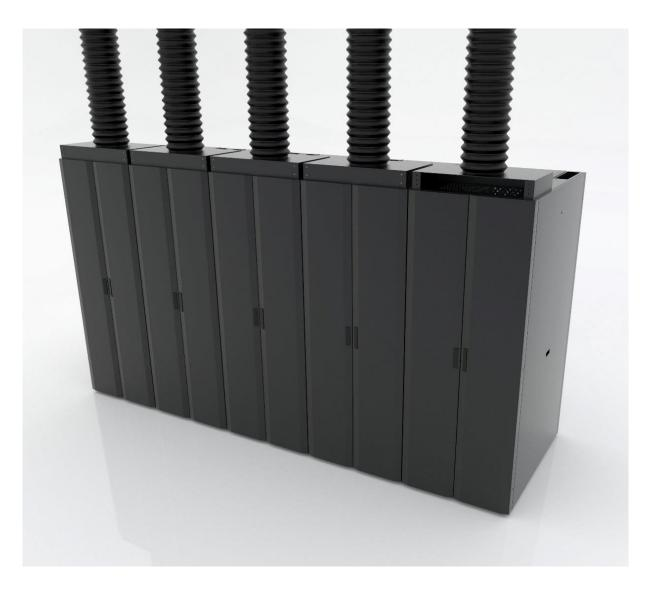
When enclosures in a row do not align with ceiling tiles and the overhead duct system, the DL Custom High Capacity Flexible Duct Chimney Kit is an ideal solution! The kit comes with a ceiling panel to be installed in the drop ceiling. The energy efficiency offered can be further enhanced when the chimney is connected to a ducting system which returns hot air to the CRAC unit (creating a closed loop system)
